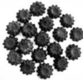
Gambar 2. Pellet Besi Hasil Proses Microwave
