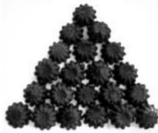
Gambar 3. Pellet Besi Campuran Silika Hasil Proses Microwave
